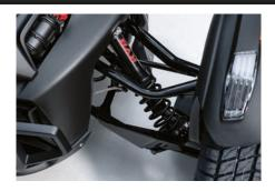
**FULL KYB† HPG SHOCKS** Front and rear KYB† HPG shocks with remote adjusters and 1 inch of extra suspension travel to optimize your ride and improve comfort.
