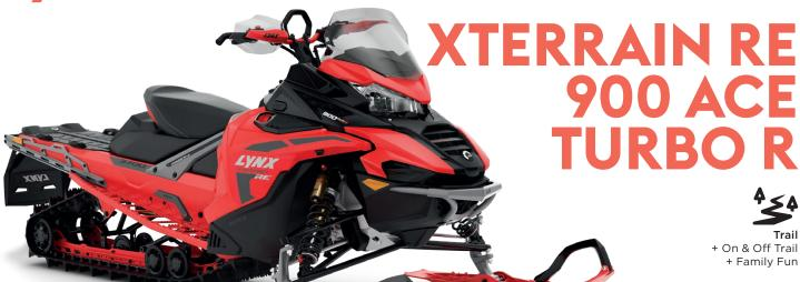
**ROTAX® ENGINE** 900 ACE Turbo R Liquid-cooled, four-stroke D.O.H.C., turbocharged **Engine details** Cylinders Displacement 899.0 cc Bore 74 mm Stroke 69.7 mm Maximum engine speed 7900 RPM Carburation EFI Recommended fuel type Unleaded Minimum octane 95 Fuel tank 37 liters
